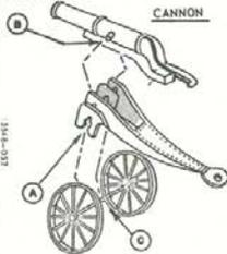
TO ASSEMBLE FIELD CANNON, SPREAD CARRIAGE (A) AND INSERT PINS (B) OF BARREL INTO HOLES OF CARRIAGE. NEXT SNAP CARRIAGE ON AXLE (C).
