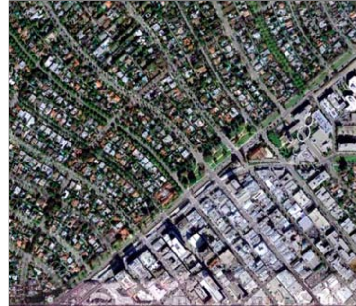
8. An interconnected network of multi-modal thoroughfares: Streets within the neighborhood form a connected network, which disperses traffic by providing a variety of vehicular and pedestrian routes to any destination. The interconnected network thus offers multiple entry and exit points for each neighborhood and creates a series of easily navigable and human-scale blocks.
