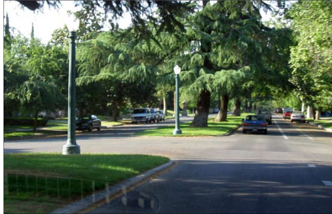
Avenue (A) A moderately-paced 2 to 4-lane section (sometimes with a median) with off-peak parking, typically for longer distances, often connecting neighborhoods or districts. Streetscapes are as varied as the contexts through which the Avenue passes.
