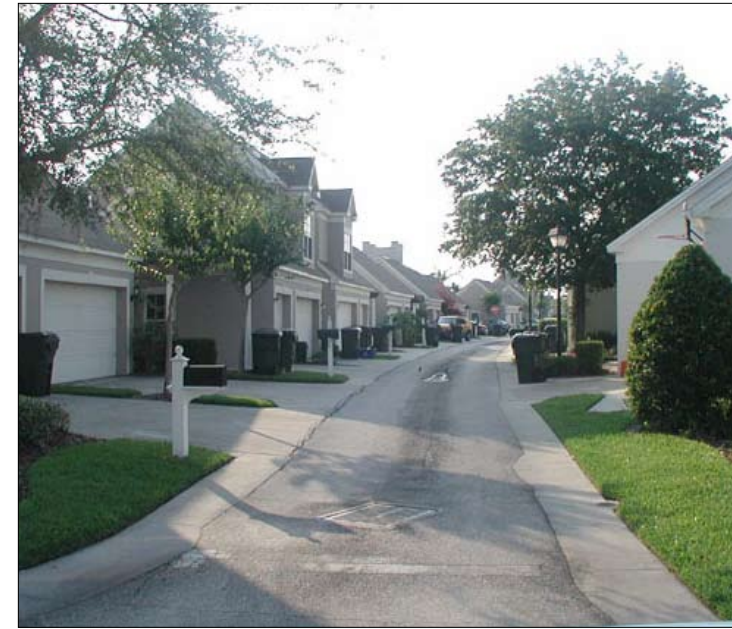
11. Parking is provided at the rear of buildings: Parking lots and garage doors rarely front the street. Parking is usually accessed by alleys. Large parking lots and large numbers of cars should not dominate the urban landscape; instead, they should be secondary to the public realm and the built fabric.
