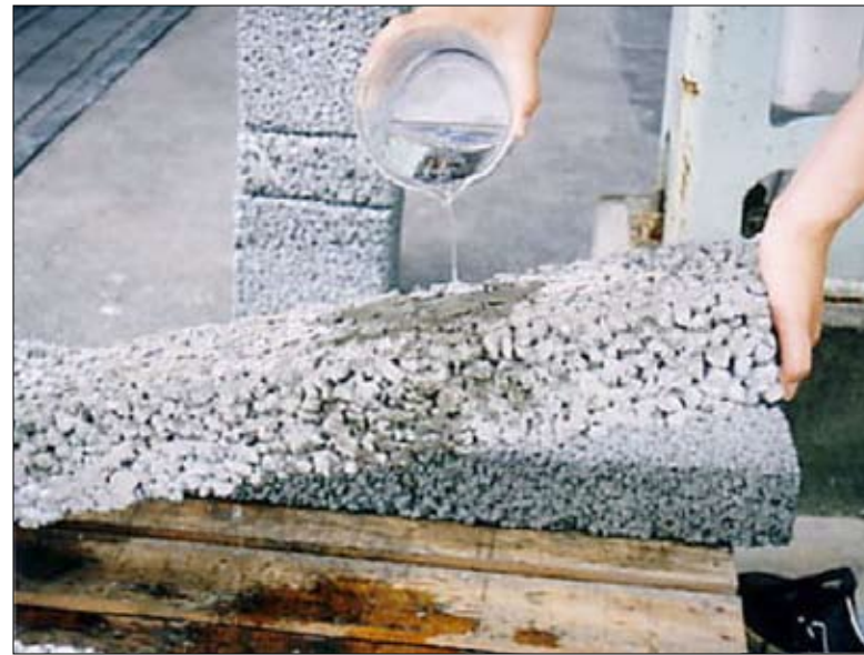
Above: Permeable concrete has the appearance of a solid surface while allowing natural drainage to occur.
