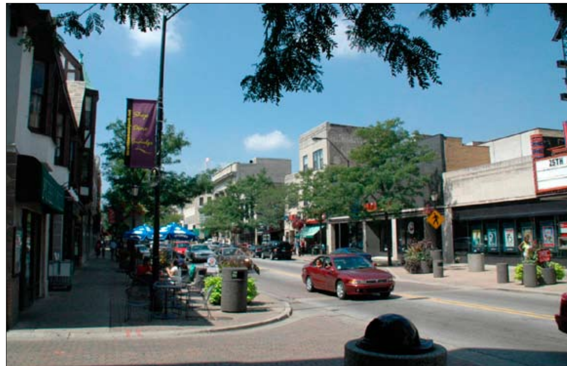
Main Street (M) A slow, 2-lane section with on-street (parallel or diagonal) parking, typically for 2 to 5 blocks, with a very intense and mixed-use streetscape.
