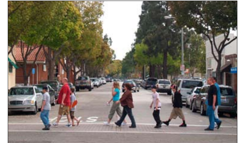
A crosswalk can be defined by striping and/or a change in paving material.
