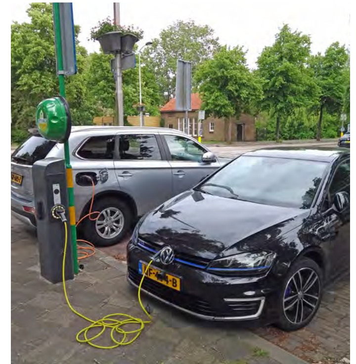
Figure A2.8b: Electric vehicle charging station (Francis Flinch - Own work, CC BY-SA 4.0, https://commons.wikimedia.org/w/index.php?curid=79231008 )
