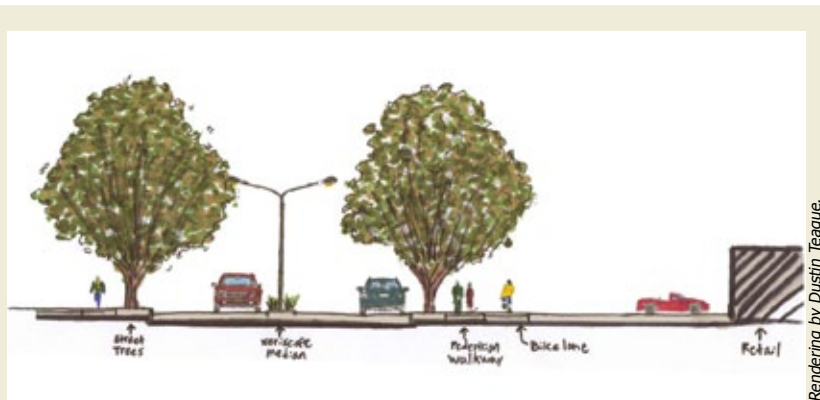
The Walzem Street cross section could be redesigned to incorporate bike lanes, wider sidewalks, and shade trees. Construction could be completed in phases.
