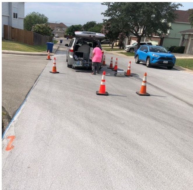
Figure 37. Tire marks causing discoloration over treated site at Rebeccas Trail.
