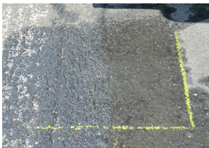
Figure 6. Marking from the CT Meter to align DF Tester in the same location.
